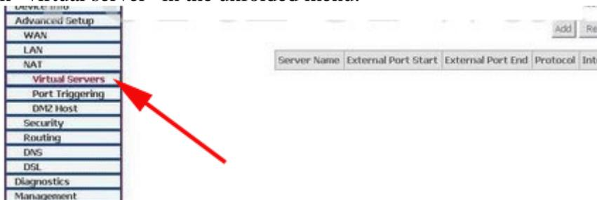
4. fill “80” under the right **port start** or **port end**, **Server IP address** fill "192.168.1.50", protocol select "TCP/UDP"OR” “TCP” , finally don’t forget click under “save/apply”
